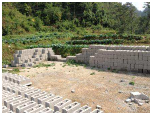
Figure 3.16. Drying and stacking of concrete blocks at the plant near Chalal Ganeshthan
