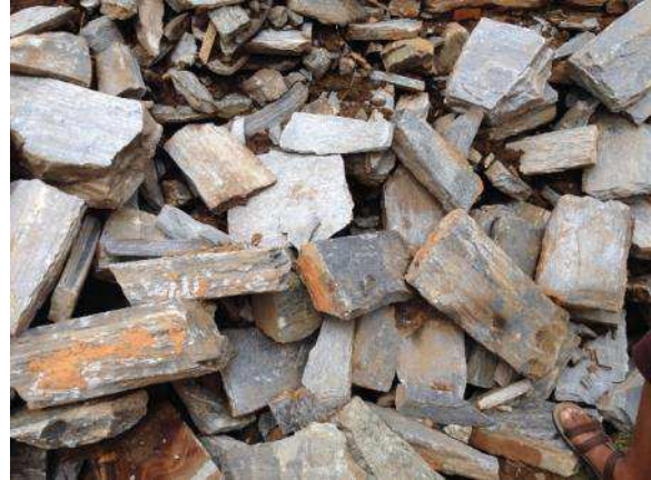
Figure 3.9. Stones used for wall construction, Maneshwor, Sindhupalchok
