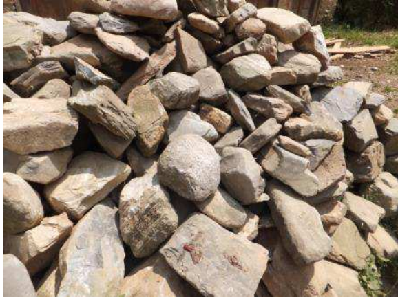
Figure 3.8. Stones used for wall construction, Dhungharka, Kavrepalanchok
