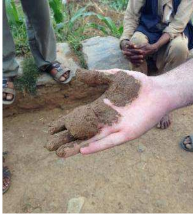
Figure 3.12. Local showing how Chimte mato binds when mixed with water.
