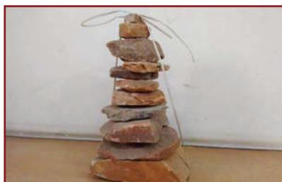
Stones in a stack when tied with a string do not fall when shaken. Stones in a wall in the house when tied with wires do not dislodge during an earthquake.
