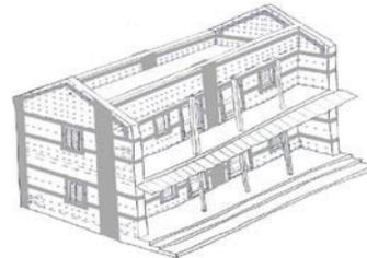
4. GI wire cross-links installed through full thickness of all the walls for anchoring the Vertical Containment Reinforcement wires in the spaces not covered by belts and splints.
