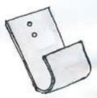
7. Install steel hooks at eave level to support the stone tiles along their bottom edge to prevent sliding and uplifting by wind.
