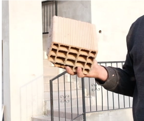
FIGURE 19 Hollow clay bricks mainly used as non structural material in infilled walls in RC Frames.
